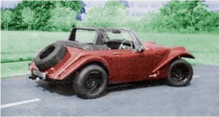
The Arkley was a way of recycling your rusty/damaged Spridget, as long as the damage/rust did not affect the main structural members, and was designed by John Britten in 1970 and produced at his works at Arkley in Barnet, hence the name. Basically the front wings, nosecone and bonnet, are removed and discarded (!), the "cycle" wings are reduced in size and the Arkley fibre
